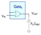
$$t_{PROP} = t_{REF} \sum_{k=1}^{n} f_k \qquad f_k = g_k h_k$$
