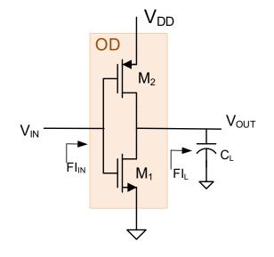
Scaling widths of ALL devices by constant (W<sub>scaled</sub>=WxOD) will change "drive" capability relative to that of the reference inverter but not change relative value of  $t_{\rm HL}$  and  $t_{\rm LH}$
