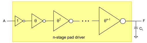
Example: Design a pad driver for driving a load capacitance of 10pF with equal rise/fall times, determine  $t_{PROP}$  for the pad driver, and compare this with the propagation delay for driving the pad with a minimum-sized reference inverter.
