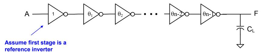
Need to determine the number of stages, n, and the OD factors for each stage to minimize  $t_{PROP}$ .
